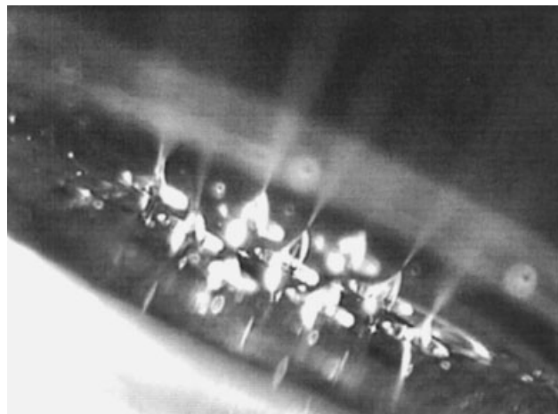
FIGURE 13. Photograph of nine electrospray Taylor cones on a microfabricated emitter array. Charging of the ESI solution is more efficient with multiple Taylor cones than with just one [Reprinted from Tang et al., Anal Chem , 2001, 73:1568–1663 with permission of American Chemical Society].
